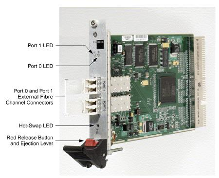
Figure 2.1 LSI7202CP CompactPCI Host Adapter
